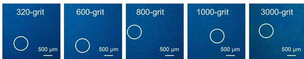
Supplementary Figure 20. Different grits (320-, 600-, 800-, 1000-, and 3000-grit sandpaper) of sandpaper imprint images of PCN-128 film (Scale bars: 500 \mu\text{m} ).
