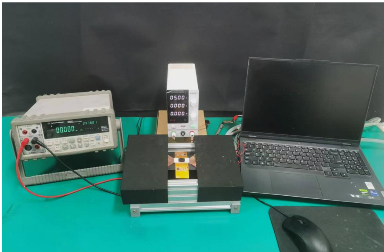
Supplementary Figure 3. Optical image of the experimental setup for characterizing the transverse thermoelectric performance of the flexible device.
