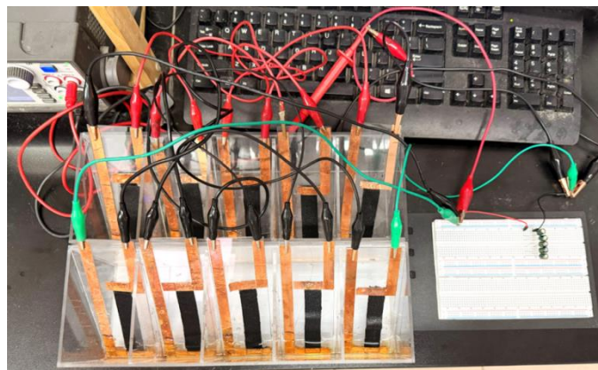
Supplementary Figure 31. Photograph for the series and parallel experiments of ten power generation devices to charge capacitors.
