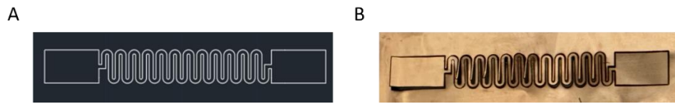
Supplementary Figure 1. Serpentine resistive heater fabrication: (A) serpentine resistive pattern designed in AutoCAD; (B) serpentine resistive element obtained by laser cutting (Photographed by the authors).
