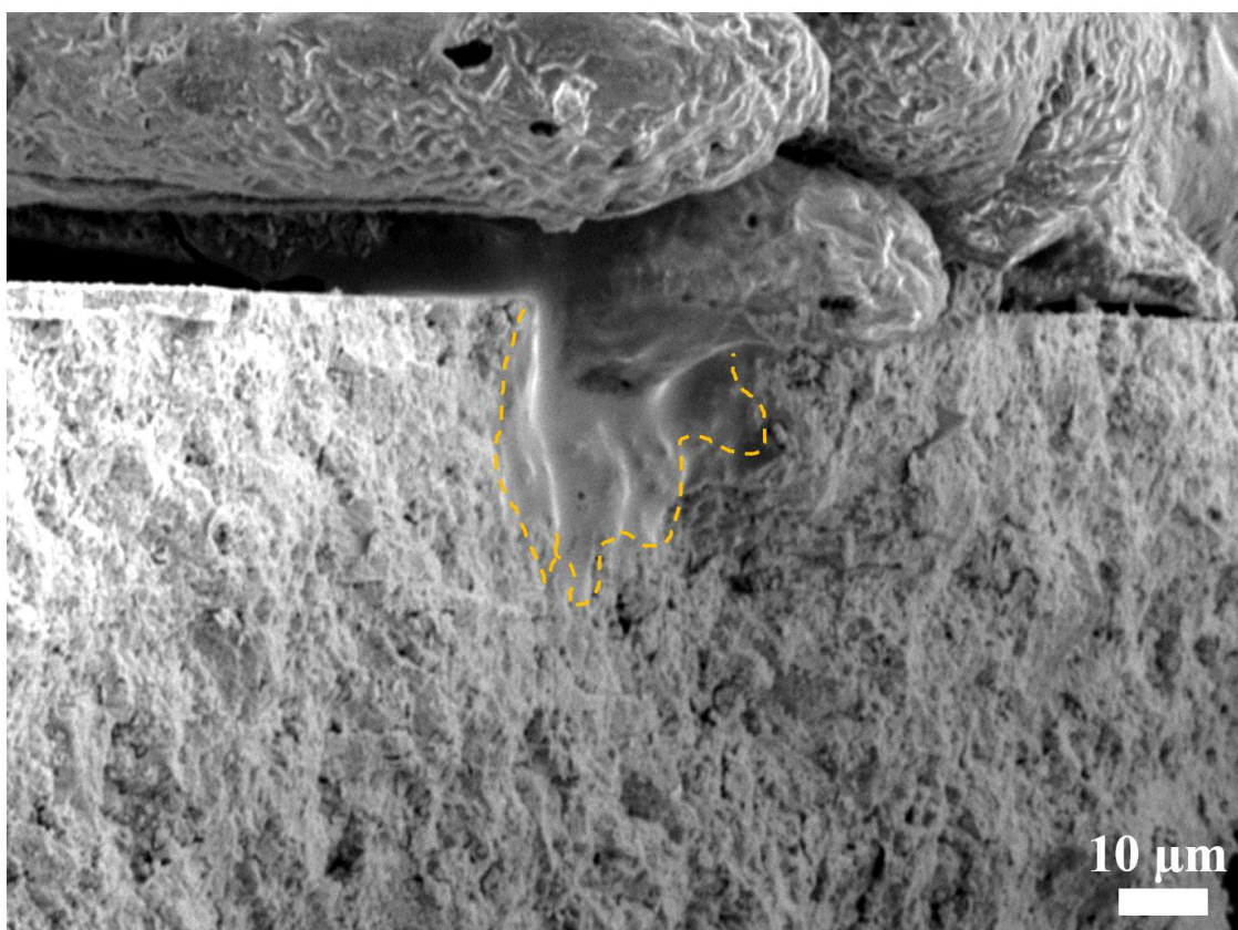
Figure S5. Cross-sectional SEM image of the NSS electrolyte after 50 cycles in a disassembled NFMO|NSS|Na cell at 55 °C.
