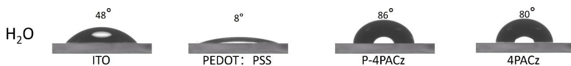
Supplementary Figure 9. H 2 O contact angles on: bare ITO; ITO/4PACz; ITO/P-4PACz; ITO/PEDOT:PSS.
