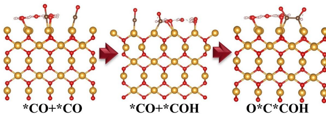
FigureS6. Structures of the reaction intermediates (*CO, *COH, and O*C*COH) of 4HB-H 2 O on a Cu 2 O (100) electrode.
