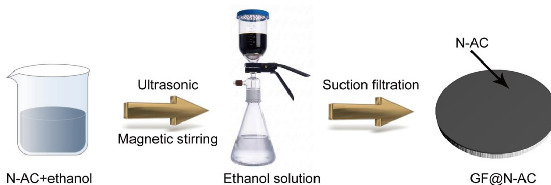
Figure S1 Schematic diagram of GF@N-AC separator synthesis process.
