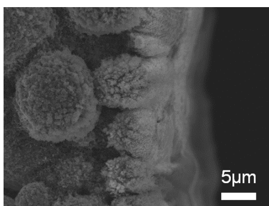
Figure S6. High-magnification SEM images of the laser-structured NCM cathode near the hole.
