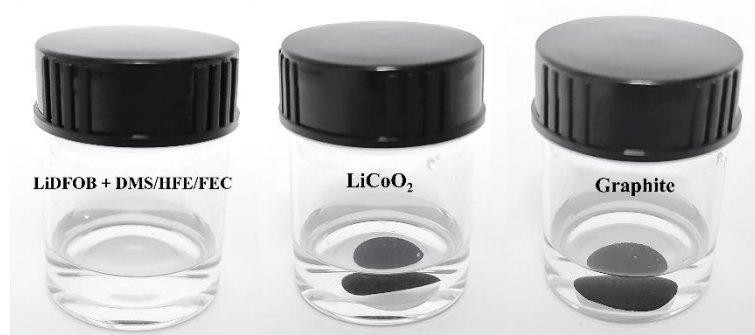
Figure S30. Visual observation of LiDFOB+DMS/HFE/FEC electrolyte at -20°C.
