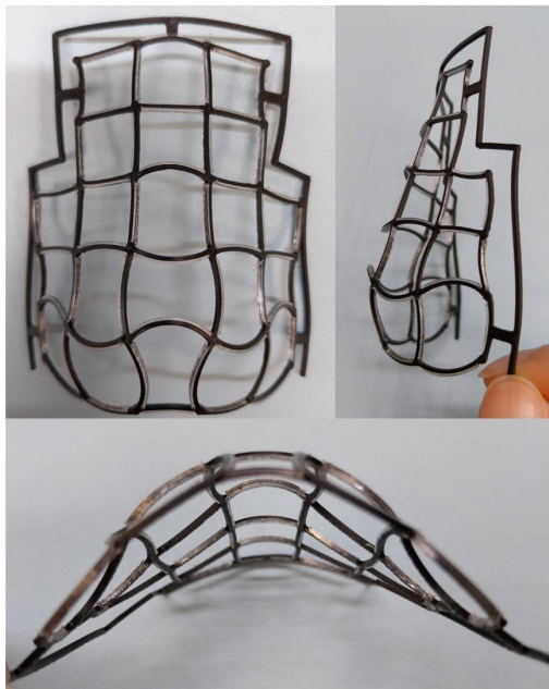
Supplementary Figure 5. Long-term stability of 3D thin shells following thermal activation. The line matrix images in (A) and (B) are separated by 15 months, and the curve matrix images in (C) and (D) are separated by 8 months, demonstrating sustained structural stability.
