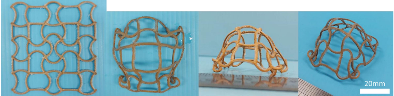
Supplementary Figure 6. Heterogeneity of the curve matrix. A curve matrix is considered heterogeneous when curvature angles vary within the same row or column. This variation arises from differing elongations of individual rib units. Rib units with greater elongation are constrained by neighboring units with lesser elongation, resulting in out-of-plane (three-dimensional) deformation.
