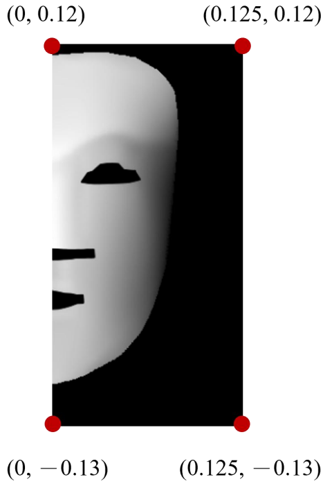
Supplementary Figure 21. Boundary range of each shell in the XY coordinates was fixed for (A) mask and (B) nose, with depth values defined based on the height range of the thin shell. Units in meters.
