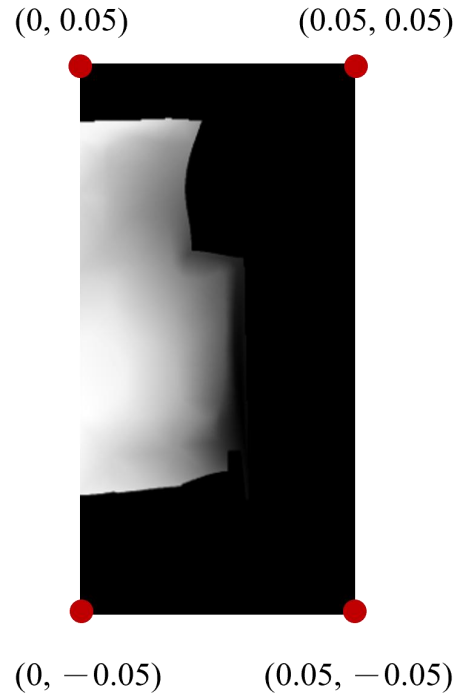
Supplementary Figure 21. Boundary range of each shell in the XY coordinates was fixed for (A) mask and (B) nose, with depth values defined based on the height range of the thin shell. Units in meters.
