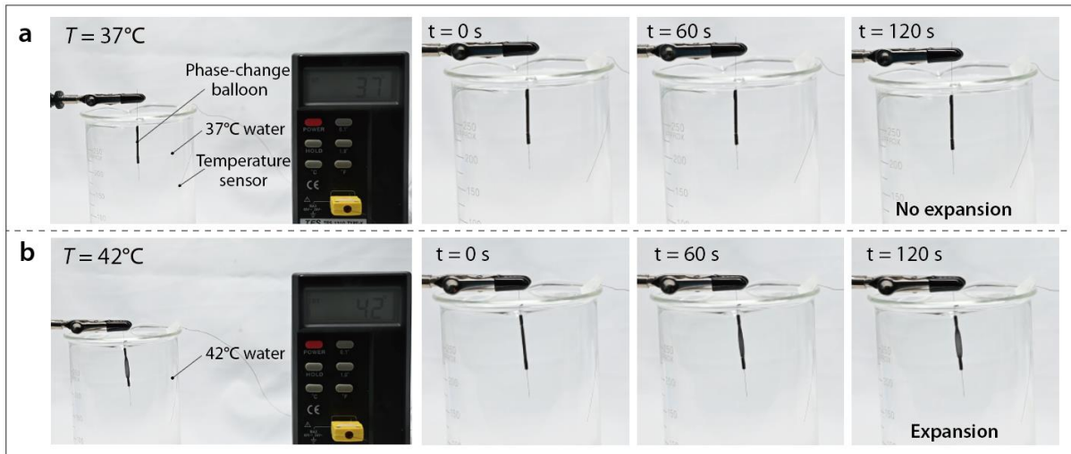
Supplementary Figure 4. Evaluation of balloon expansion behavior at different environmental temperatures. (a) At 37 °C (below the phase transition threshold), the fluid remains in a stable liquid phase and the balloon does not expand. (b) At 42 °C (reaching the phase transition temperature), the liquid-to-gas transition is triggered, leading to balloon expansion (Photographed by the authors).
