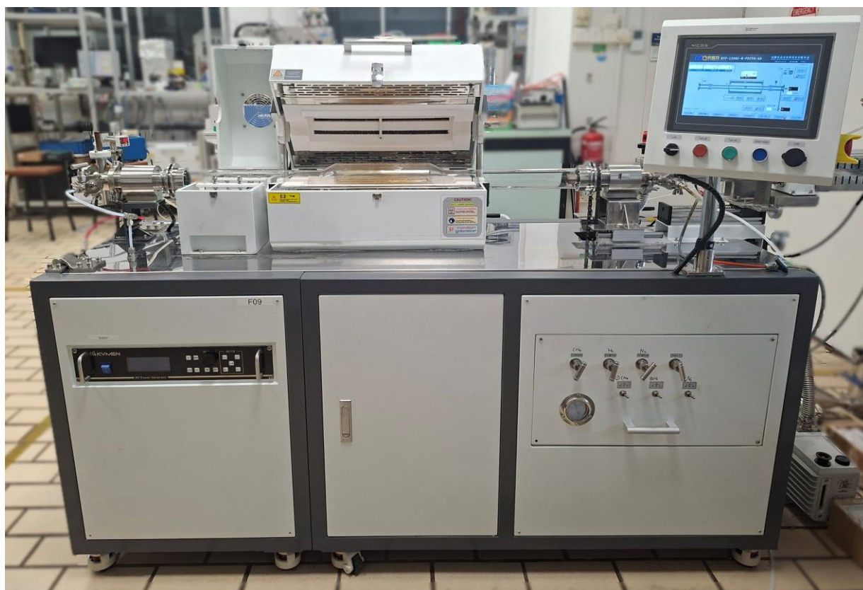
Fig. S2. Photograph of the rotary-bed reactor used for CDM experiments with furnace opened, showing the quartz tube.
