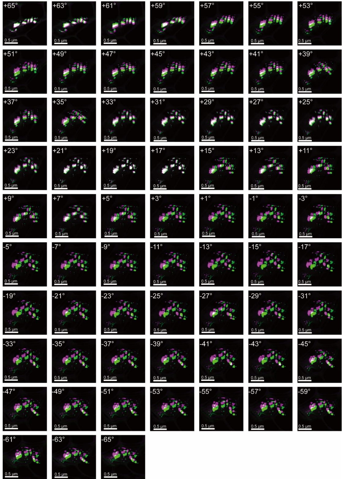
Supplementary Figure 5. Differential map of tilt series acquired by rapid/conventional-acquisition method. Using conventional acquisition images as the reference, differential map displays intensity-deficient regions in red, intensity-enhanced regions in green, and intensity-overlapping areas in white for the rapid-acquisition images.
